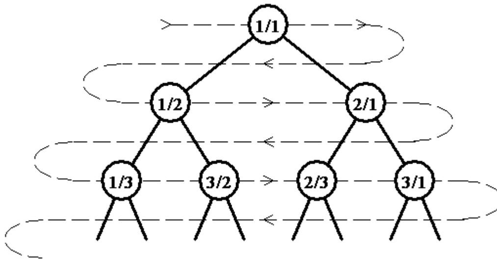
A rational sequence is defined by doing a level order (breadth first) traversal of the tree (indicated by the light dashed line). So that:
