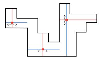
Given an x-monotone rectilinear polygon, write a program to compute the minimum number of sensor units required to completely monitor the polygon.
